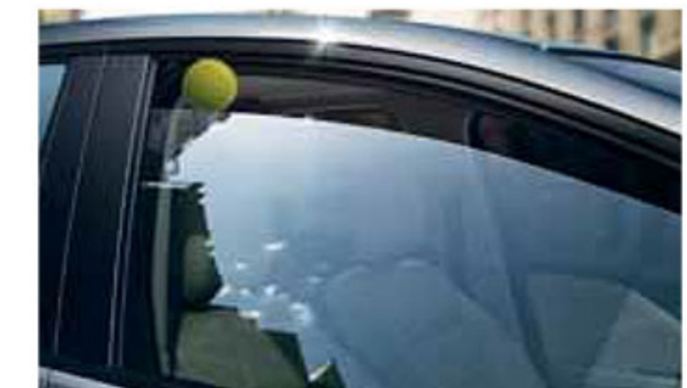
Driver Side Pinch Guard & Auto Down Function
